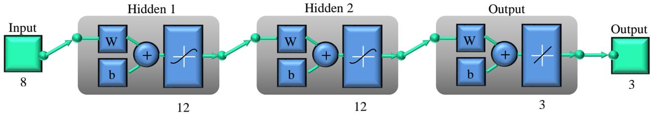
Fig. 6 The best MLPNN structure for printing applications
