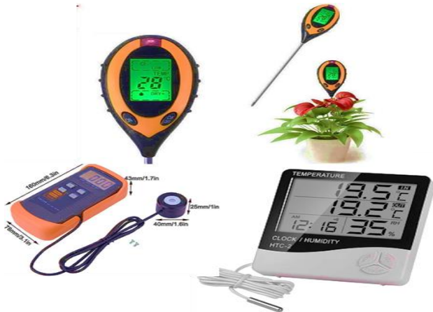
Fig. 12 Conventional instruments for nursery monitoring
