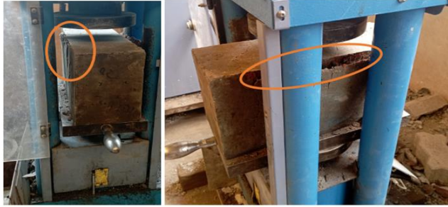
Fig. 12 Local failure of concrete
