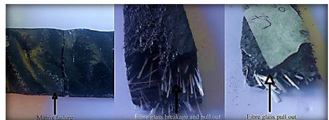
Fig. 7 Failure mode of composites
