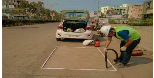
Fig. 5 Collection of dry accumulation using a vacuum cleaner
