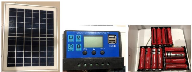
Fig. 3 Solar panel, charge controller, and battery ultrafine
