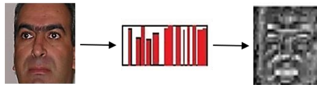
Fig. 5 LBP face generation from the input face image
