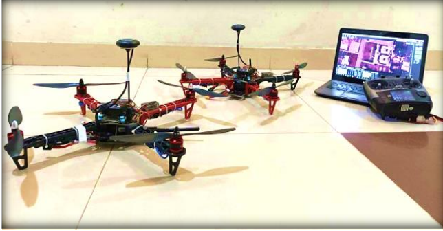
Fig. 4 Experimental setup used for path loss prediction
