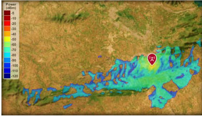
Fig. 2 Antenna coverage for transmitter placed in the residential area
