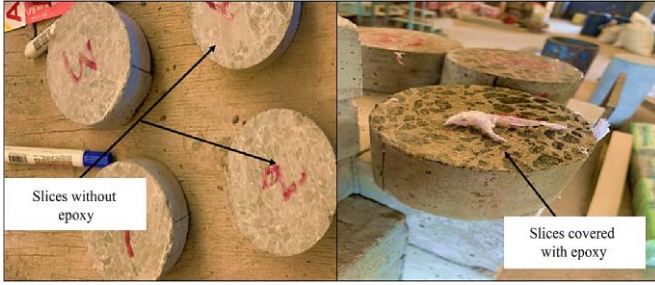
Fig. 2 Concrete slices for testing
