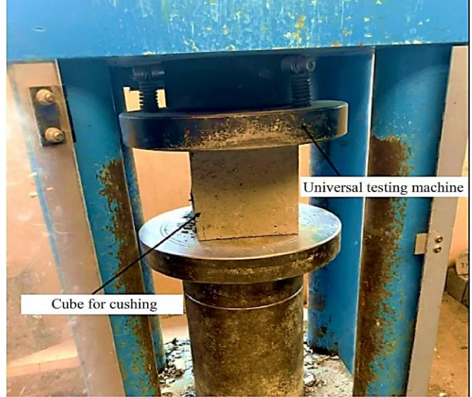
Fig. 6 Crushing machine setup
