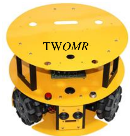
Fig. 1 Mobile robot using omnidirectional wheels
