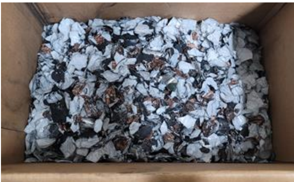
Fig. 1 The shape of waste LFP battery that has passed through a shredder
