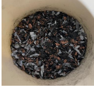
Fig. 3 Photo of the waste LFP battery shreds after screening and classification
