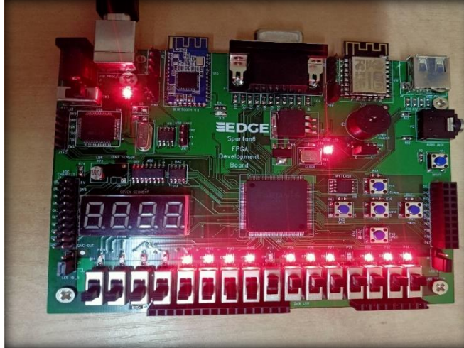
Fig. 17 Hardware output of the hamming encoder
