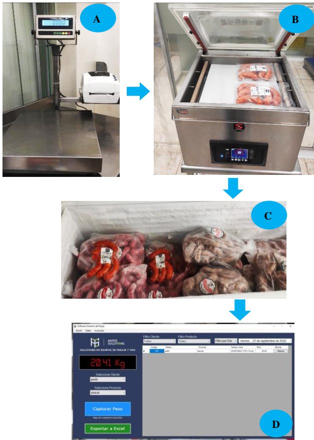
Fig. 8 Final process of the weighing system.
