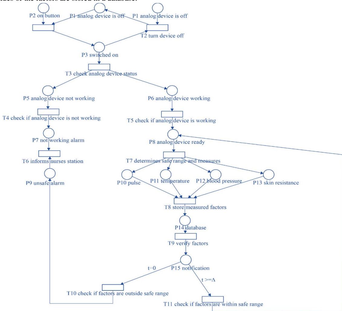
Fig. A.2.2 PN of Patient monitoring system drawn after analysis and correction for consistency and completeness is done.
