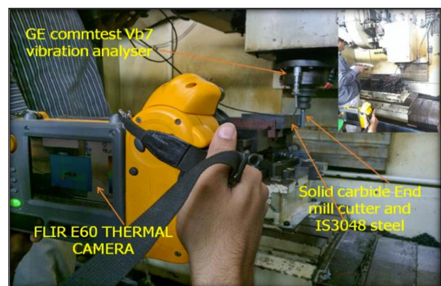
Fig. 1 Drilling IS3048 Steel in an Experimentation Setup
