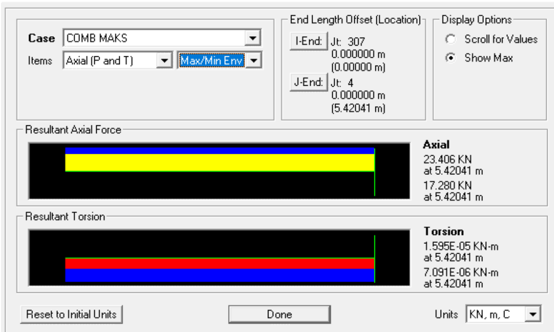
Fig. 27 Axial force. Double elbow steel profile 40.40.4
