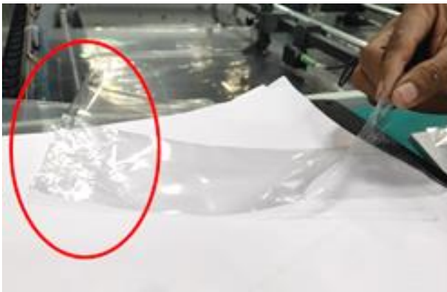
Fig. 3(a) Wrinkles in plastic bags - Defect
