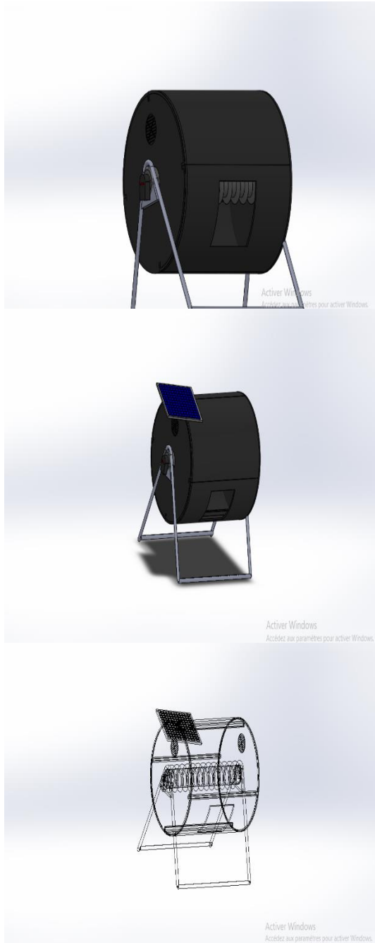
Fig. 1 Design of the self-contained rotating composter with shredding shaft by SolidWorks.
