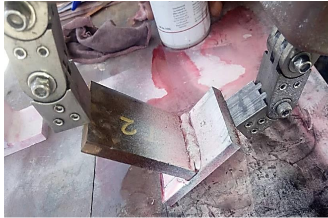
Fig. 5 Magnetic particle inspection
