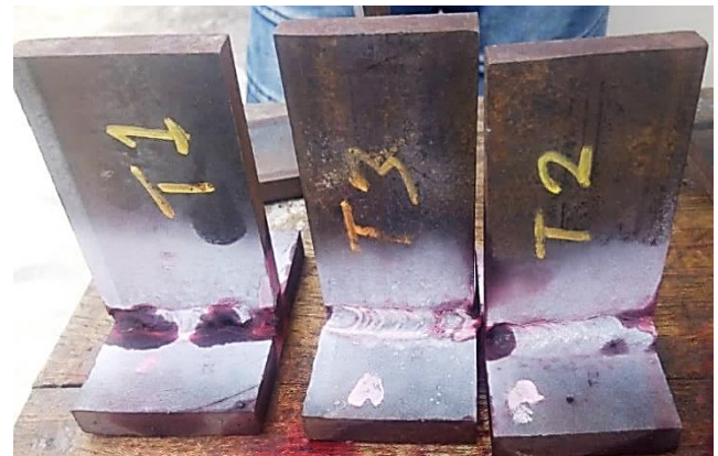
Fig. 4 Dye penetrant inspection results of tee joint
