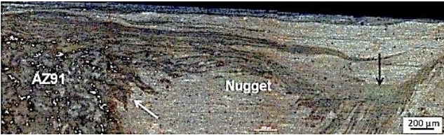
Fig. 10 Micro structure taken at the cross-section of welding process at high magnification dissimilar welding process Az-91/Az-31
