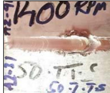
Fig. 12b The weld was made at 1400rpm at 50 tool traverse speed with dissimilar welding Az91/Az31 alloy
