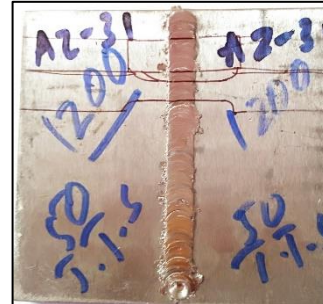
Fig. 5a The weld made at 1200rpm at 50 tool traverse speed with similar welding Az31 alloy
