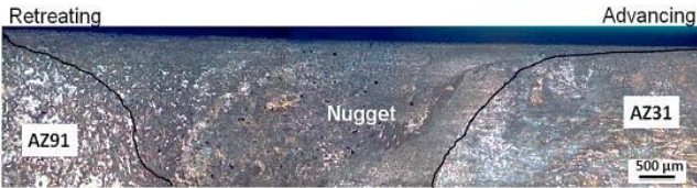
Fig. 9 Micro structure taken at a cross-section of welding process at low magnification dissimilar welding process Az-91/Az-31
