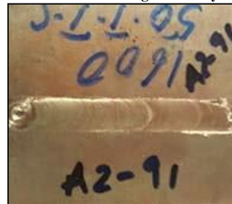
Fig. 7c The weld was made at 1600rpm at 50 tool traverse speed with similar welding Az91 alloy
