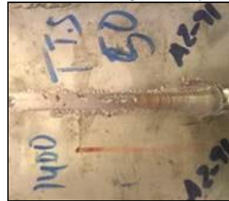
Fig. 7b The weld was made at 1400rpm at 50 tool traverse speed within stir welding Az91 alloy
