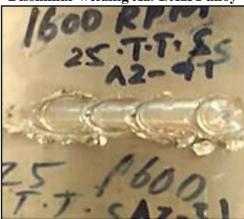
Fig. 8b The weld was made at 1400rpm at 25 tool traverse speed with dissimilar welding Az91/Az31 alloy
