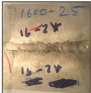
Fig. 6c The weld was made at 1600rpm at 25 tool traverse speed with similar welding Az91 alloy
