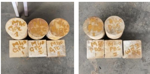
Fig. 3 GPC & NC specimens with chloride attack
