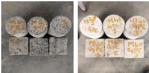
Fig. 1 GPC & NC specimens with acid attack
