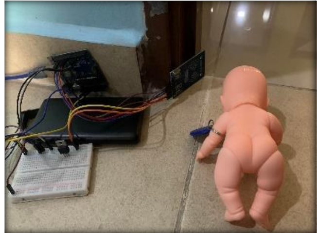
Fig. 5 Wearable RFID tag, and RFID reader
