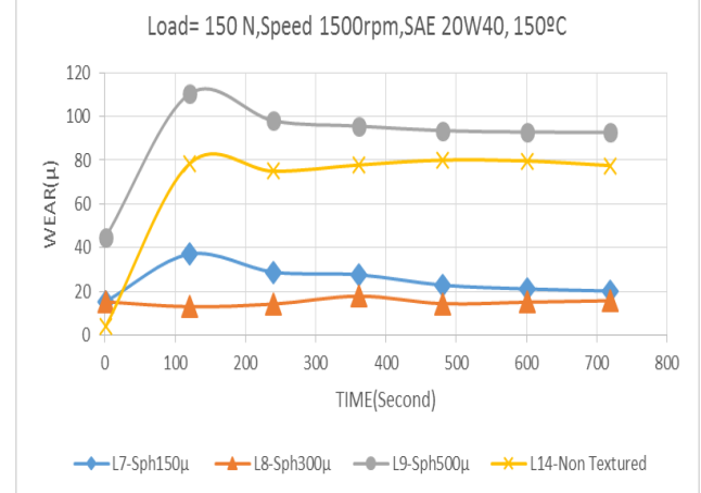
Fig. 11 Wear of liner sliding with spherical dimple shape piston ring specimen at 150N and 1500 rpm
