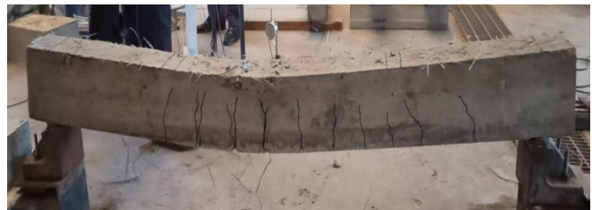
Fig. 16 Failure Patterns of the Control Beam (Top) and Modified Beam (Bottom) with Shear Reinforcement
