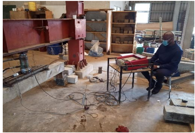
Fig. 3 Four-Point Load Test Setup
