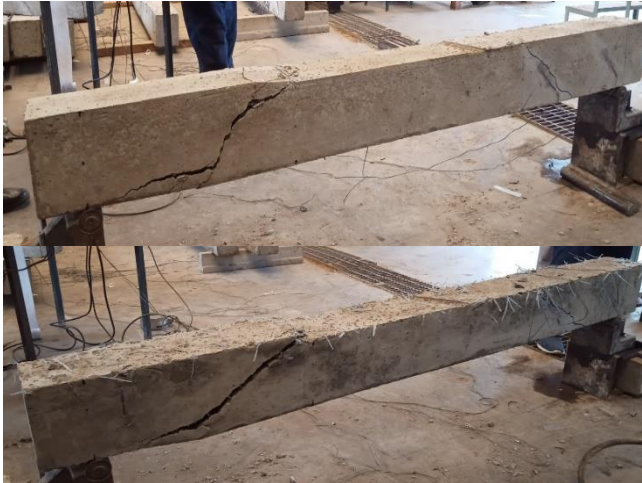
Fig. 14 Failure Pattern of Control Beam (Top) and Modified Beam (Bottom) without Shear Reinforcement
