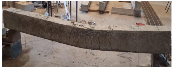
Fig. 15 Crack Distributions at Failure
