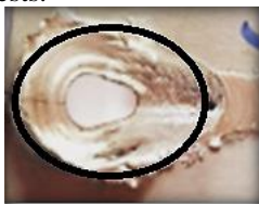
Fig. 3(a) Material peeled while under stir process and also a hole through the top to the bottom
