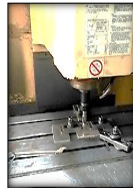
Fig. 1(d) CNC machining set up for FSW process
