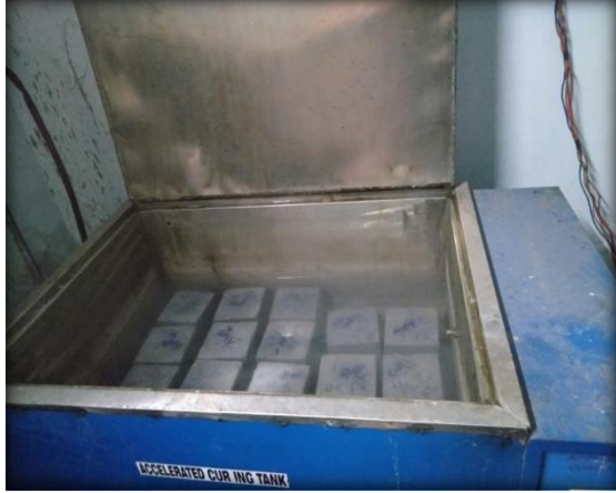
Fig. 1 (c) Immersed specimens in an accelerated curing tank for boiling
