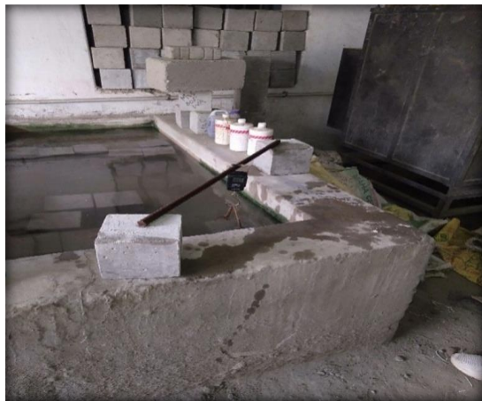
Fig. 1(d) Specimens under suspension in water by a wire
