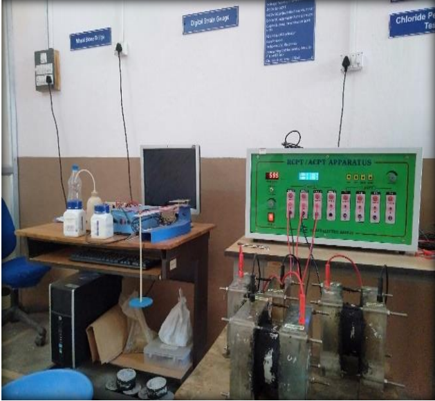
Fig. 9 RCPT Set up in the laboratory
