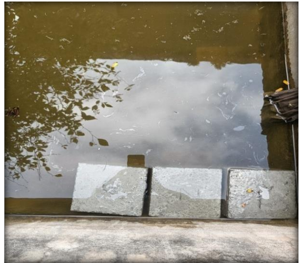
Fig. 1 (b) Immersed specimens in curing tank for saturation
