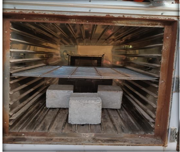
Fig. 1 (a) Oven-dried specimens
